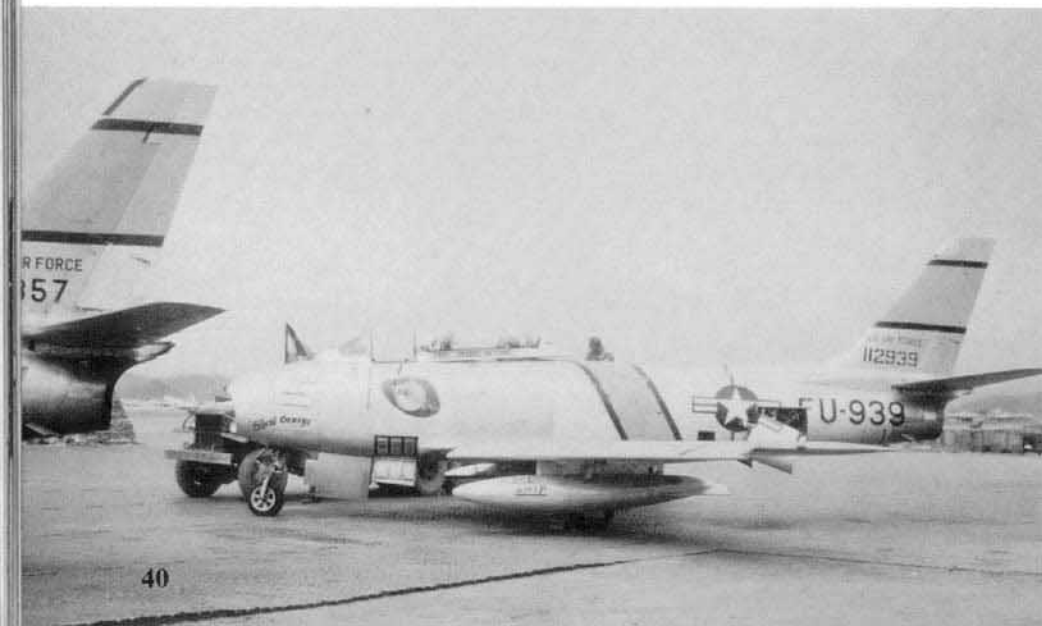
Silent George was an F-86F-10 of the 336th FIS, flown by CAPT George Love. The aircraft was about to depart Taegu for Tsuiki, Japan for retrofit with the hard edge wing. NAA sent some fifty wing kits to Japan for installation on F-86Fs flown by aces. (Alan Fine)
