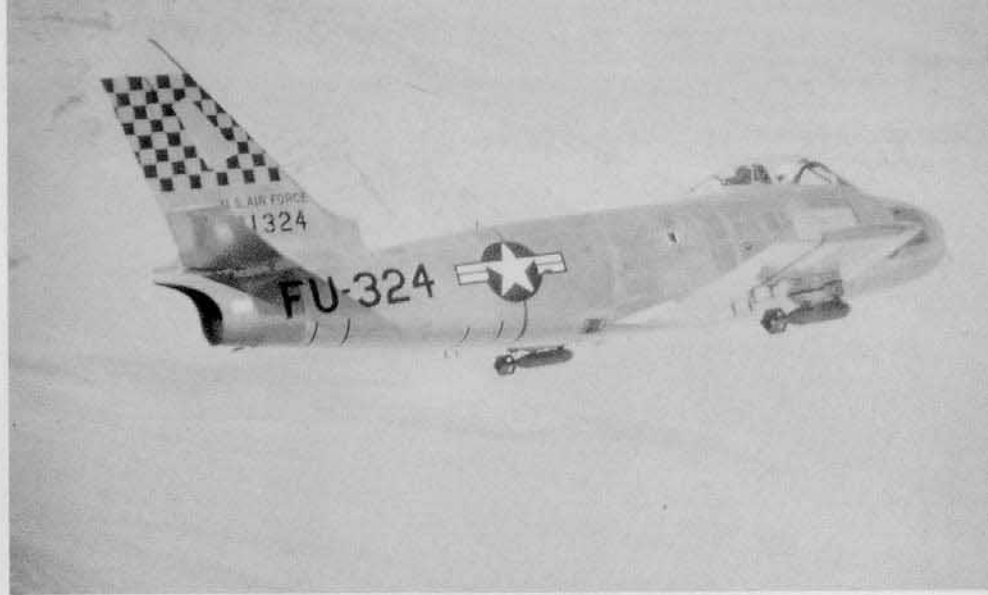
The primary training unit for Sabre pilots was the Fighter School at Las Vegas Air Force Base (now Nellis AFB), Nevada. This F-86A carried a Black and Yellow checkered tail. The F-86A-5 could carry a pair of underwing fuel tanks or bombs, such as these 250 pound Blue practice weapons. (David Menard)
