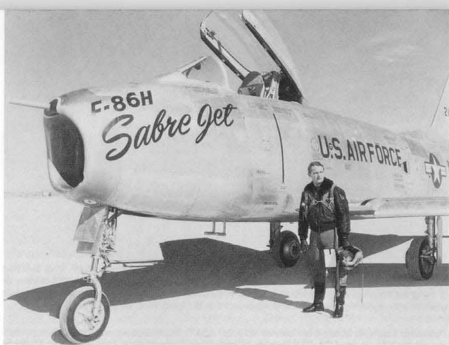
North American Chief Test Pilot "Wheaties" Welch stands by the nose of the F-86H prototype (52-1975). The F-86H was to have solved all the complaints about the Sabre program, since it had much more power and a cannon armament. (NAA)
