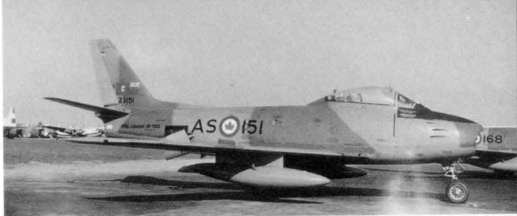
The Canadair equivalent to the F-86F was the Sabre Mk 5, although the Canadian built aircraft were powered by an Orenda 10 engine in place of the General Electric J47. This Sabre Mk 5 was assigned to No 416 Squadron, RCAF based at Grostenquin. (Brian Baker)
