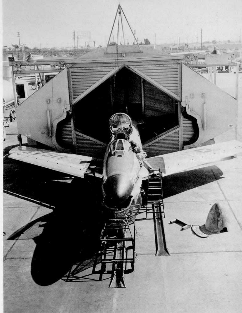
An F-86D in the engine test shed at the NAA facility in Inglewood. A complete test of all systems, including the engine, was required before an aircraft was accepted by the Air Force. The sliding doors on the shed were shaped to fit the F-86D fuselage, sealing in most of the engine noise. (Fernando Silva)
