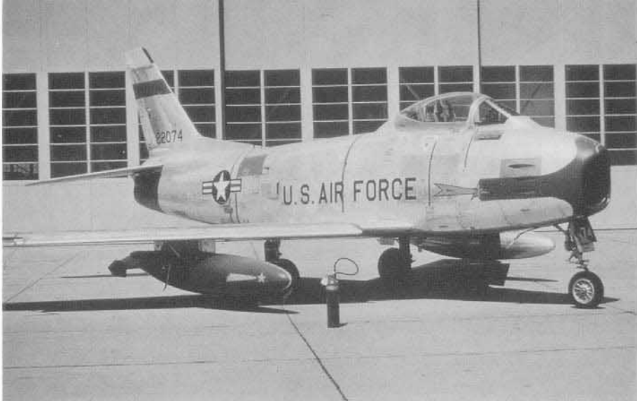
This F-86H-1 was bailed to Lockheed for use as a chase aircraft for the F-104S and A-12 programs during the late 1950s and early 1960s. The nose, tail and drop tank colors are Red with the Yellow Lockheed "star" marking. (JEM Slides)
