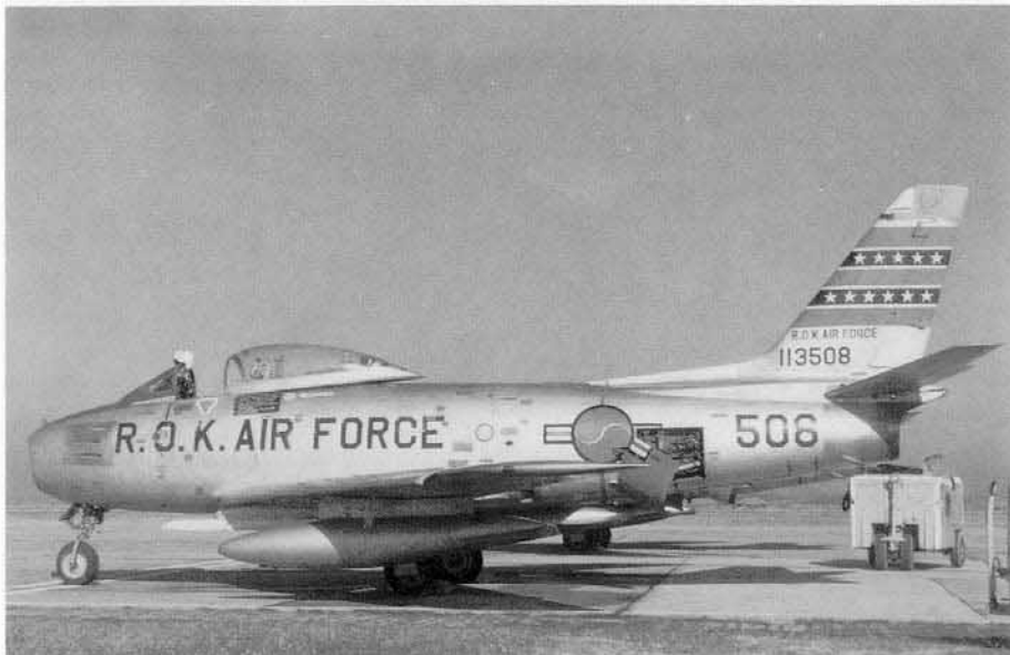
The Republic of Korea Air Force (ROKAF) was given a number of Sabres following the Korean War, flying them into the 1980s. This ex-USAF F-86F-25 was retrofitted with the 'F-40' extended wing and modified to carry the AIM-9 Sidewinder air-to-air missile. (Robert C. Mikesh)
