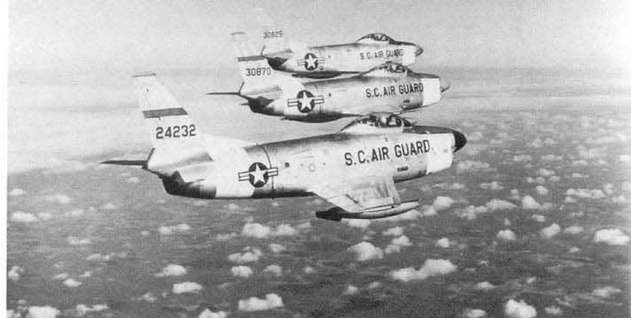
A trio of F-86Ls of the 157th FIS/South Carolina Air National Guard based at McEntire ANG Base during 1959. The F-86D block number changed one digit when the aircraft was converted to L standards. An F-86D-50 became an F-86L-51. (Jim Sullivan)
