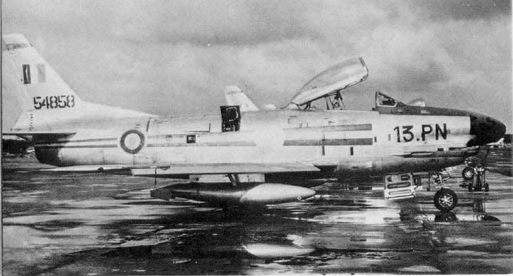
An F-86K-NF of 13 Esquadre , French Air Force during 1958. Initially F-86Ks were delivered with the standard, short-chord, short-span F-86D wing and later retrofitted with the F-40 wing. France purchased a total of sixty Fiat-built F-86Ks. (French Air Force)
