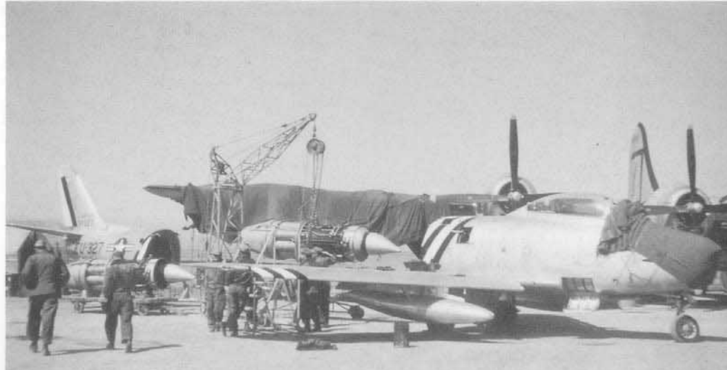
Sabre maintenance in Korea during early 1951 was usually done outdoors. These 4th FIG mechanics are doing an engine change on the Suwon ramp. The B-29 in the background was forced to land at K-13 and then turned into an open-air engine shop since there were no permanent facilities available on the field. (Irv Clark)
