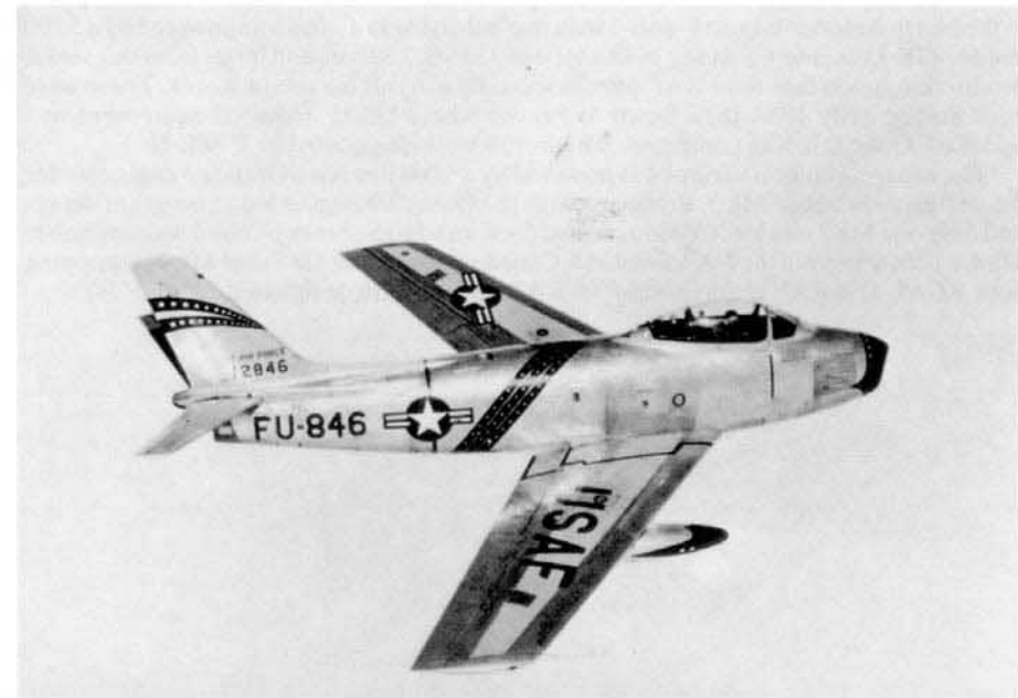
An F-86E-10 of the 42nd Fighter Interceptor Squadron based at Orchard Place AFB, Chicago (later O'Hare International) during 1953. The F-86E-10 was the first Sabre variant to use the optically flat armored windscreen. (Peter Bowers)
