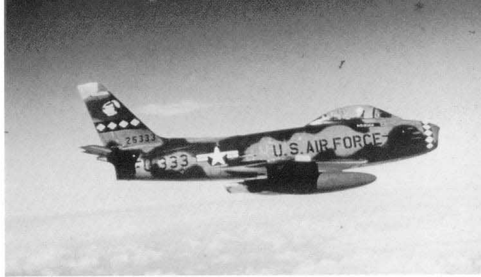
During the mid-1950s, several USAF units experimented with NATO style camouflage on both F-86s and F-84s. This F-86F of the 461st FDS is camouflaged with Medium Gray and Dark green uppersurfaces with British PRU Blue undersurfaces. The project was later cancelled and the paint stripped off. (Rob Satterfield)
