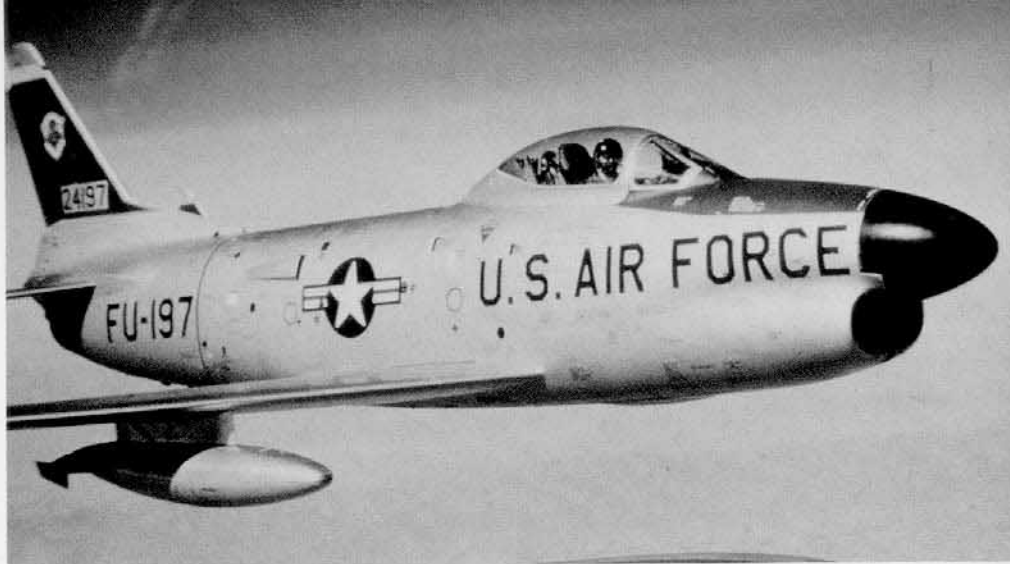
The last F-86D-45 off the assembly line went to the 456th FIS at Castle AFB, California. The D-45 introduced the drag parachute to the F-86D series which was housed in a fairing at the base of the rudder. (BGEN K.W. Bell)
