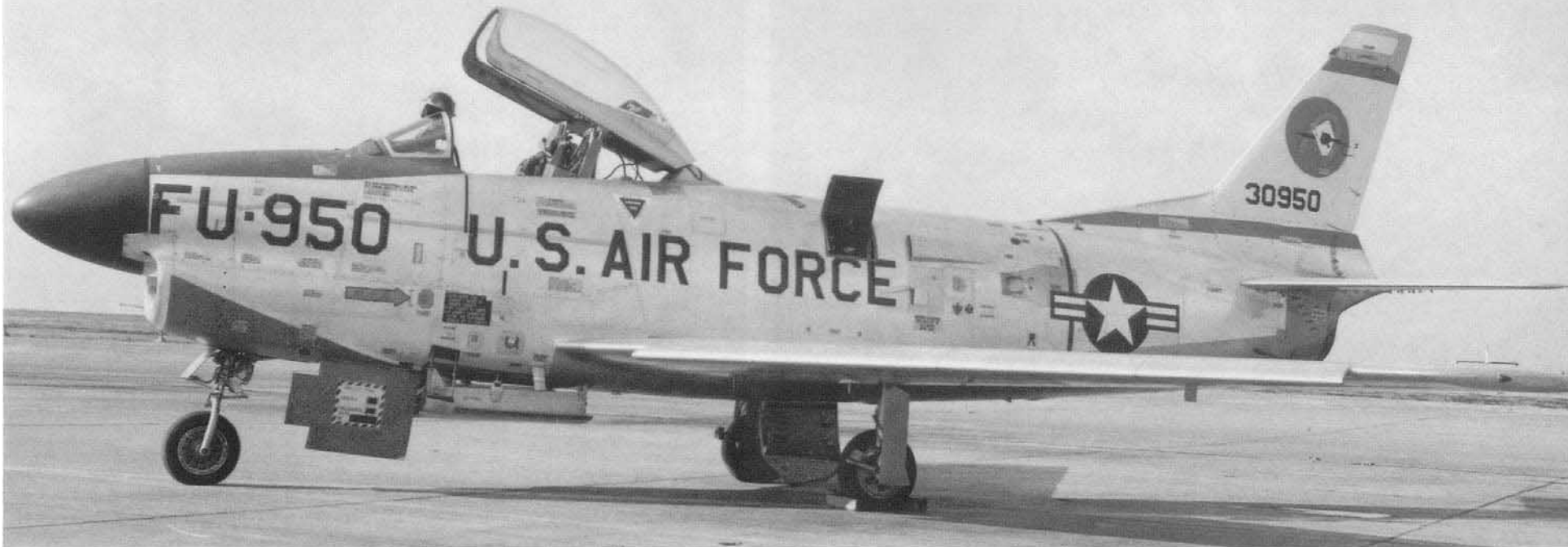
An F-86L of the 83rd FIS on the ramp at Hamilton AFB during 1958. The F-86L was a rebuilt late production F-86D with the SAGE system installed. The SAGE antenna is visible under the nose, near the rocket tray. (Jim Sullivan)
