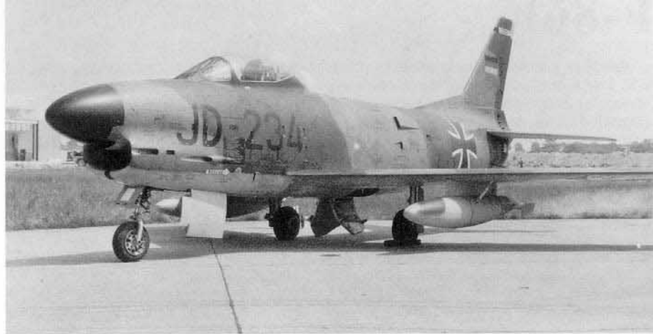
A West German Bundesluftwaffe Fiat-built F-86K of JG-74 during 1967. West German F-86Ks were painted the typical NATO tactical camouflage of Dark Green and Dark Gray uppersurfaces over Light Gray undersurfaces. (Manfred Franzke)
