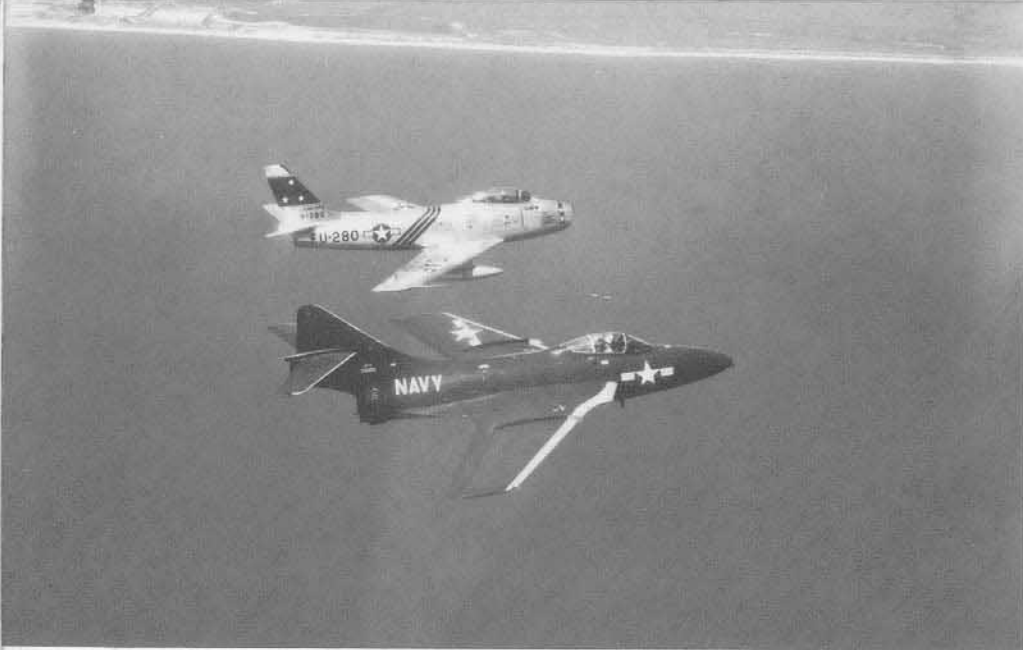
An F-86A of the 75th FIS flies formation with a Grumman F9F-6 Cougar near Long Island during 1952. The Navy had also seen the advantages of the swept wing and had contracted Grumman to develop a swept wing version of the F9F Panther. The F9F-6 Cougar was the first F9F variant with swept wings. (John M. Campbell)
