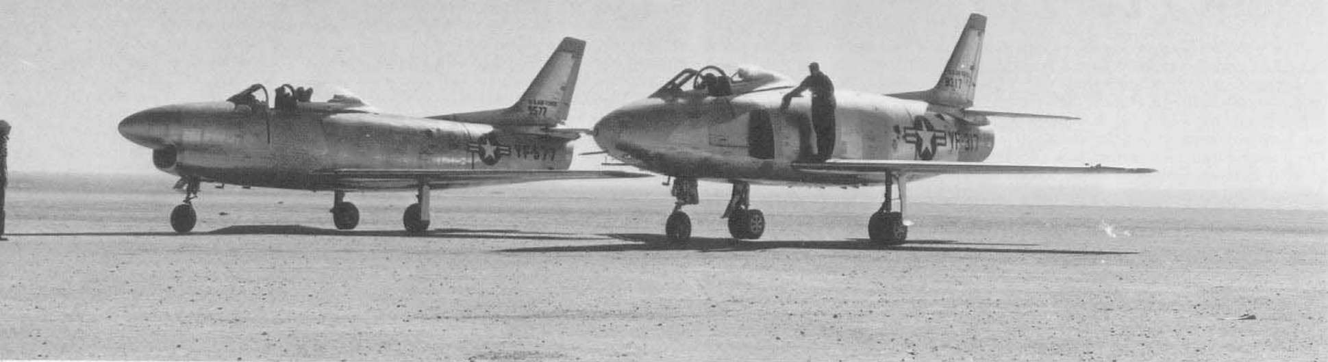
The YF-93A and F-95A share the ramp at Muroc Dry Lake Air Force Base during 1950. Both aircraft were conversions of F-86A airframes and carry service test (YF) buzz numbers on the rear fuselage. (NAA)
