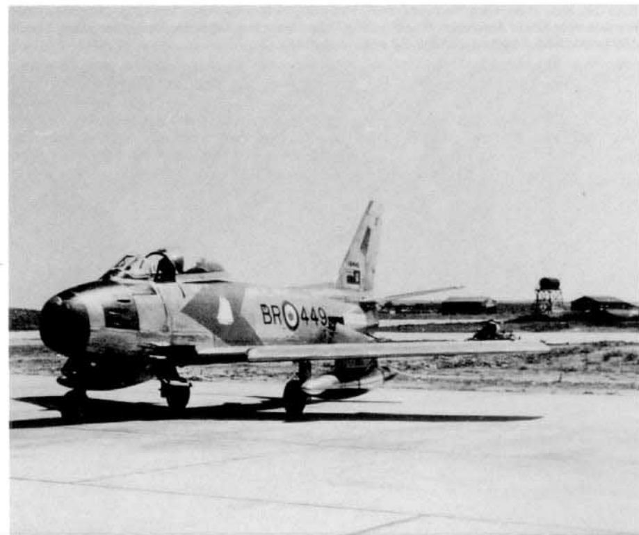
Canadair Ltd. of Canada built the F-86E in two variants: the Sabre Mk 2 and Sabre Mk 4. This Mk 2 was assigned to No 434 Squadron, Royal Canadian Air Force based at Uplands during 1952. The Sabre Mk 2 and Mk 4 were identical to USAF F-86Es. (Jan Michael Guhl)
