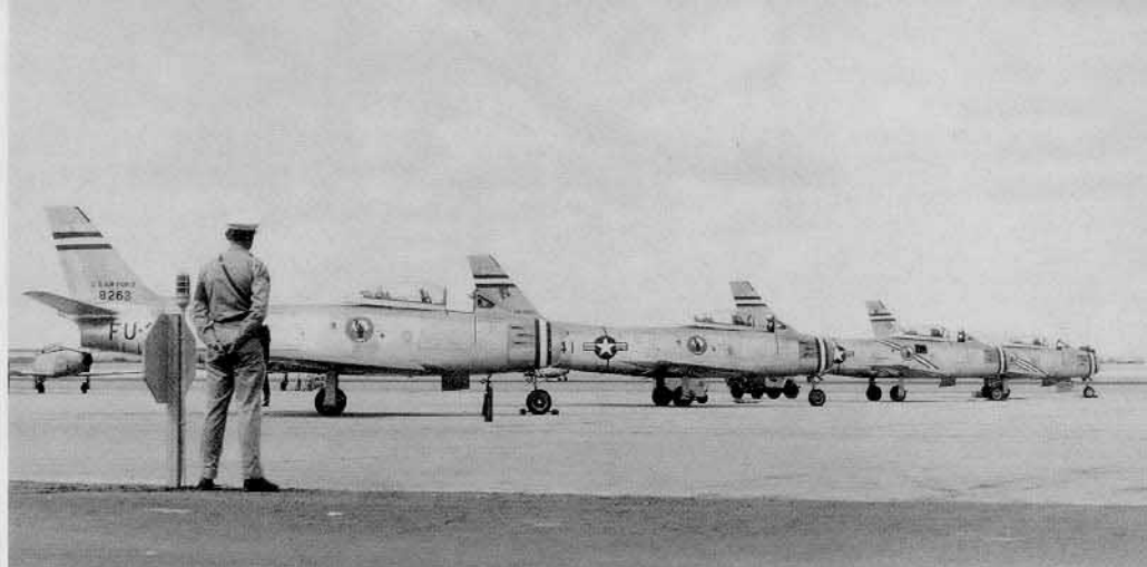
Late production F-86A-5s of the 93rd FIS/81st FIG on the flight line at Kirtland AFB, New Mexico. The 81st FIG was the third group to transition from F-80s to F-86s in 1949. Their mission was to defend the atomic bomb plant at Alamogordo, New Mexico. Late F-86A-5s had the gun port doors deleted.(NAA)
