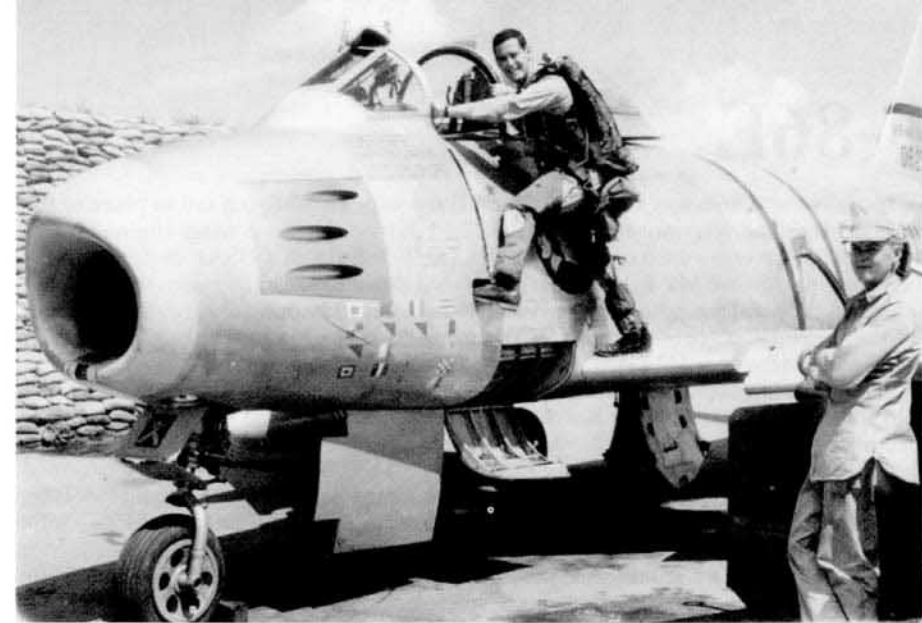
CAPT James Horowitz climbs aboard his F-86E named Slow Boat To China at Kimpo, the home base of the 4th FIW. He would later write a book about the war that was made into a popular movie titled "The Hunters." The aircraft has a V-shaped windscreen, identifying it as an F-86E-1 or E-5. (Karl Dittmers)
