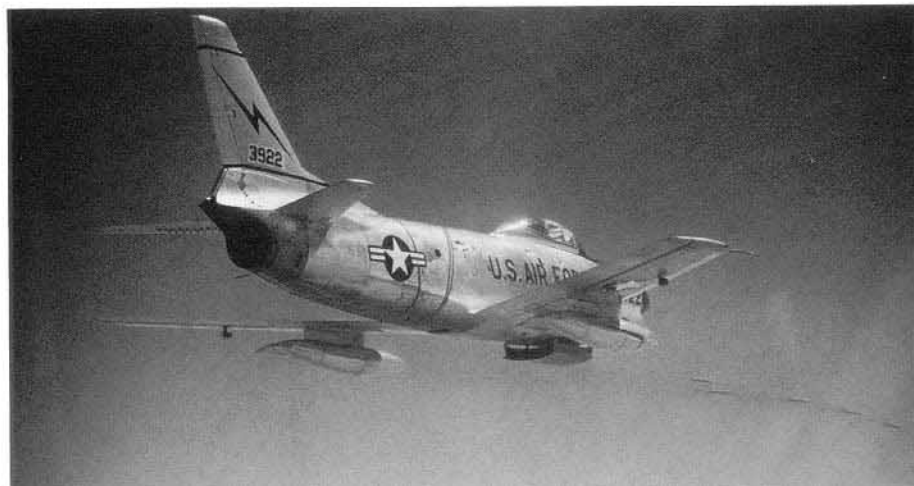
An F-86D of the 31st FIS fires a volley of 2.75 inch rockets during the 1956 Yuma Rocket Meet. For the meet, cameras were installed under each wing, outboard of the underwing fuel tanks. (Robert Wainwright)
