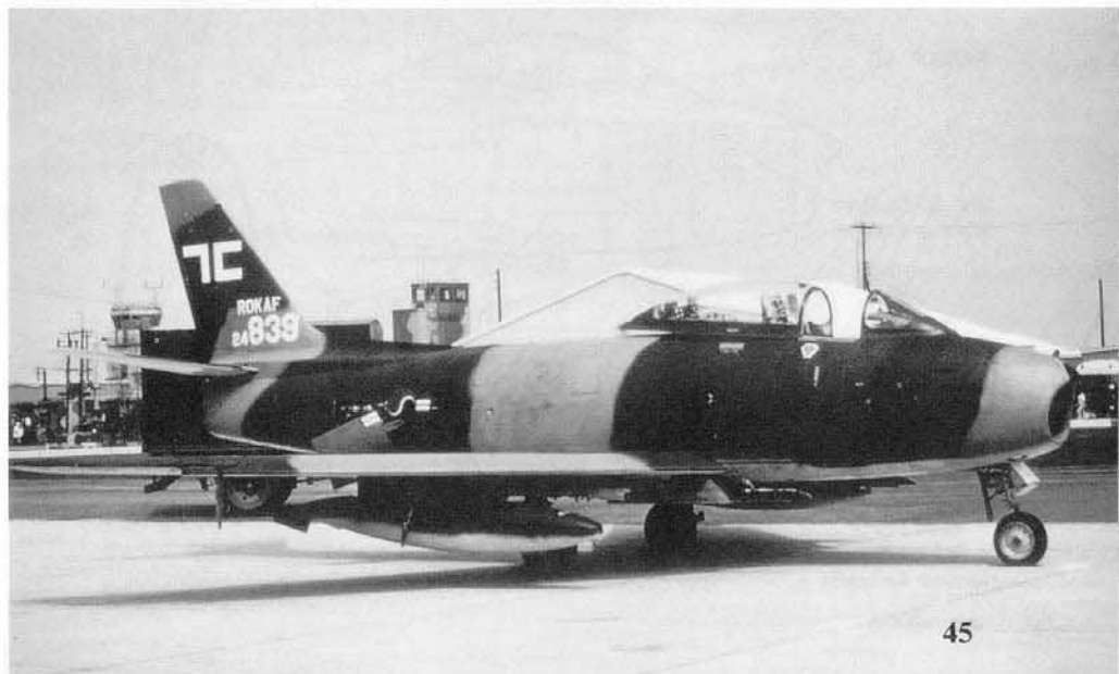
Late in their careers, Republic of Korea Air Force (ROKAF) F-86F-25 Sabres were camouflaged with Dark Green and Tan uppersurfaces over Light Gray undersurfaces. All lettering was in White. (Centurion)
