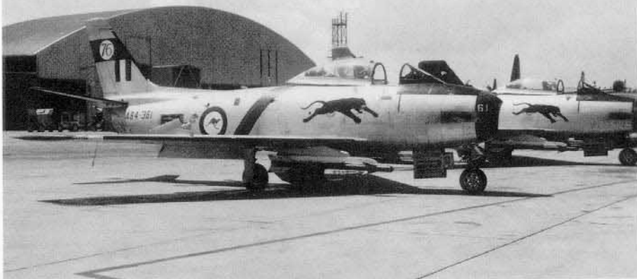
A Commonwealth CA-27 Sabre Mk 32 of 76 Black Panther Squadron, RAAF. The unit had formed an aerobatic team which flew the Sabre during the 1960s. The Mk 32 had both the '6-3' wing with fences and Sidewinder missile capability. RAAF Sabres flew combat air patrols over Thailand during the very early stages of the Vietnam War. (Brian Baker)
