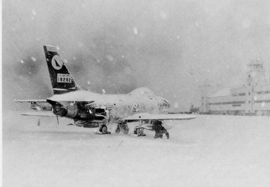
This F-86D on the snow covered ramp at Ladd AFB, Alaska during 1953 carries full Arctic markings in Red. All new aircraft and systems purchased by the USAF were sent to either Ladd AFB or to the climatic hanger at Eglin AFB, Florida for cold weather testing. (NAA)
