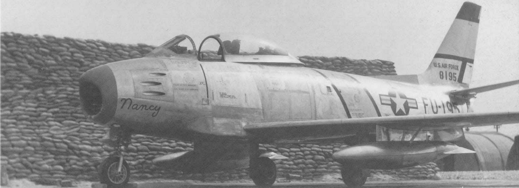
Project ASHTRAY involved conversion of at least seven F-86A-5s for the reconnaissance mission by removing their guns and adding a pair of K-22 cameras in a bulged fairing under the fuselage. Nancy was an RF-86A serving with the 15th TRS/67th TRW at K-14 in 1952. (George McKay)
