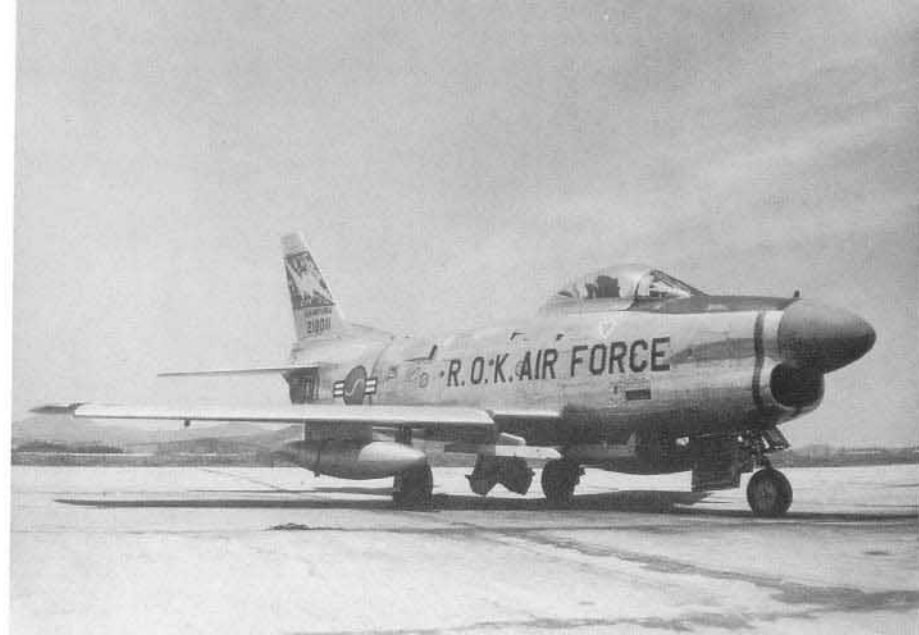
The Republic of Korea (ROK) Air Force received a number of F-86D-50s modified with AIM-9 Sidewinder air-to-air missile rails under the inboard wing panels. The small antenna on top of the nose just behind the radome is a TACAN antenna. (ROKAF)
