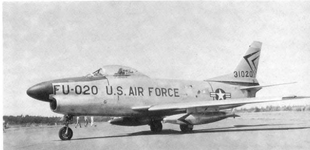
A F-86D of the Air Training Command at Yuma AFB during 1956. During 1956, the first F-86Ds were pulled from active service to begin Project FOLLOW-ON, the conversion of F-86Ds to the F-86L standard. (Brian Baker)
