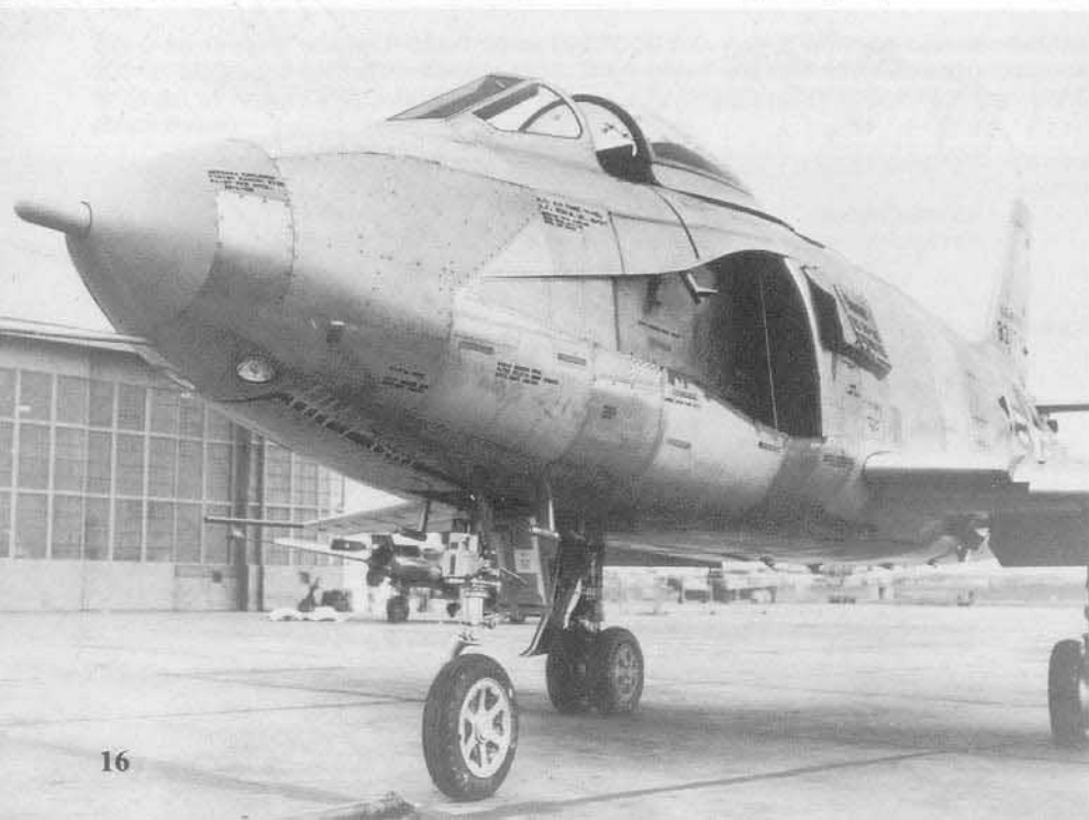
The F-86C/YF-93A was a North American Aviation project designed to create a long range, penetration jet fighter using existing Sabre technology. The F-86C/YF-93A used an 8,000 lbst Pratt and Whitney J48-P-1 engine with afterburner, had large side mounted NACA-designed flush air intakes and a dual wheeled main landing gear. (NAA)
