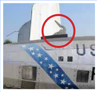
A fairly rare Cold War specimen is this RF-84K (52-7625) one of 25 modified as "parasites" to be carried by the GRB-36. Displayed outside for 20 years or more, in 2014 it showed the B-36 trapeze hook in place and extended.
