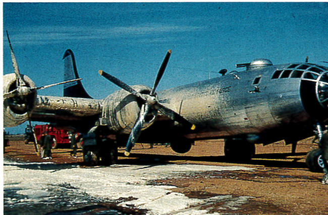
Fire retardant covers this B-29 after the bomber made an emergency landing at Kimpo in 1951. Note the No. 1 engine feathered at far left.
