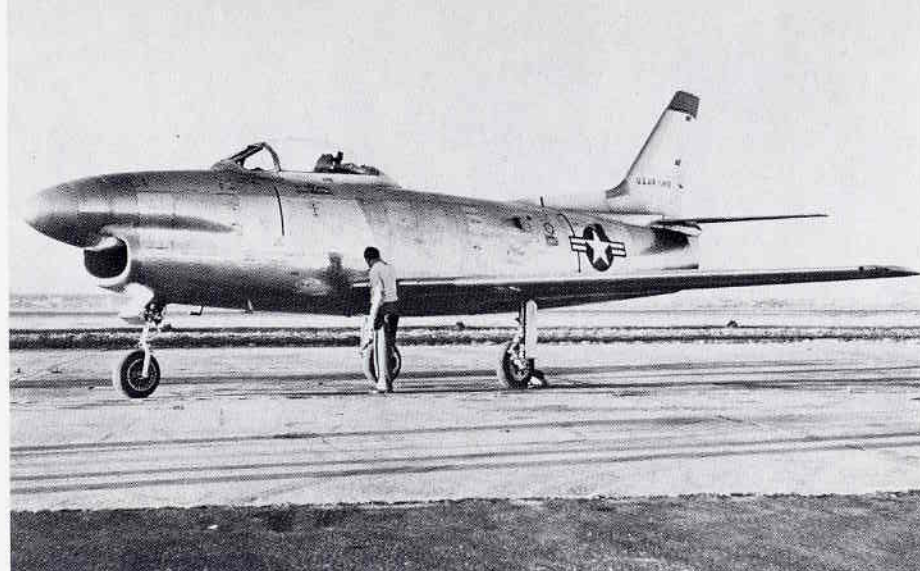
The first YF-86D, #50-577, on rollout from the North American plant in Los Angeles. Note the F-86A canopy and windscreen. [NAA]
