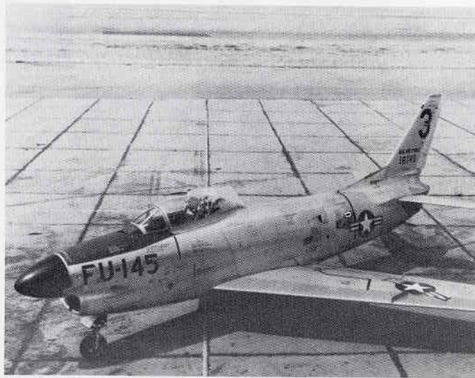
51-6145, the F-86D-35 that Lt. Col. Wm. Barnes flew to a 715 mph world record in July, 1953. Note that the aircraft has 'wing fences', a device never used on production Ds. [NAA]
