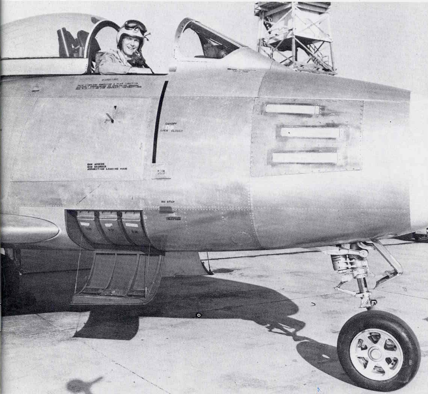
48-133 flew with the 27th FS at March AFB. Fuselage flash and upper tail stripe are yellow, lower stripe is red. Note the 206 gallon ferry tanks. [M/Sgt. David Menard]
