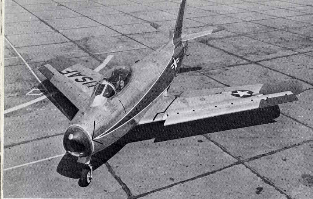
50-579 was the first F-86E. It is shown late in its life when it served as a chase plane for North American. Note the v-shape windscreen used on A-5s and early Es. [NAA]
