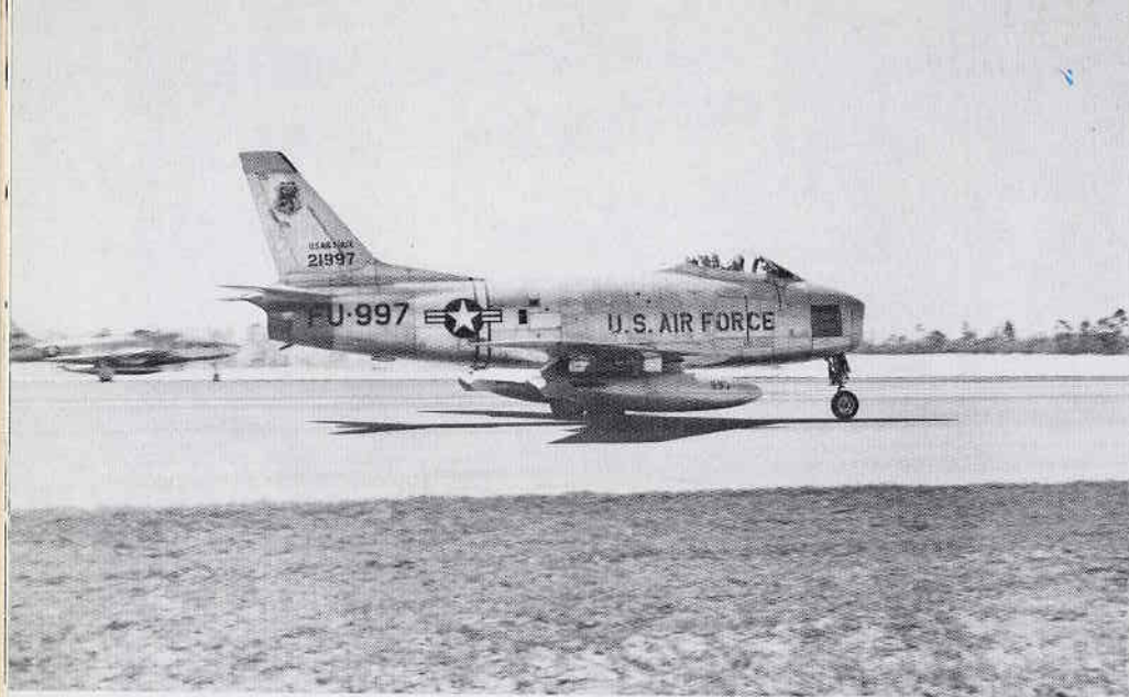
52-1997 is an F-86H-1 serving at Eglin AFB Armament Proving Center. H-1s had 6 .50 calibre machine guns instead of usual cannon armament. [USAF]
