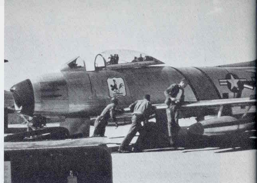
67th FBS mechanics install the new 'hard' leading edge and fences to 52-4350 at Osan AB, 1953. [Brown]
