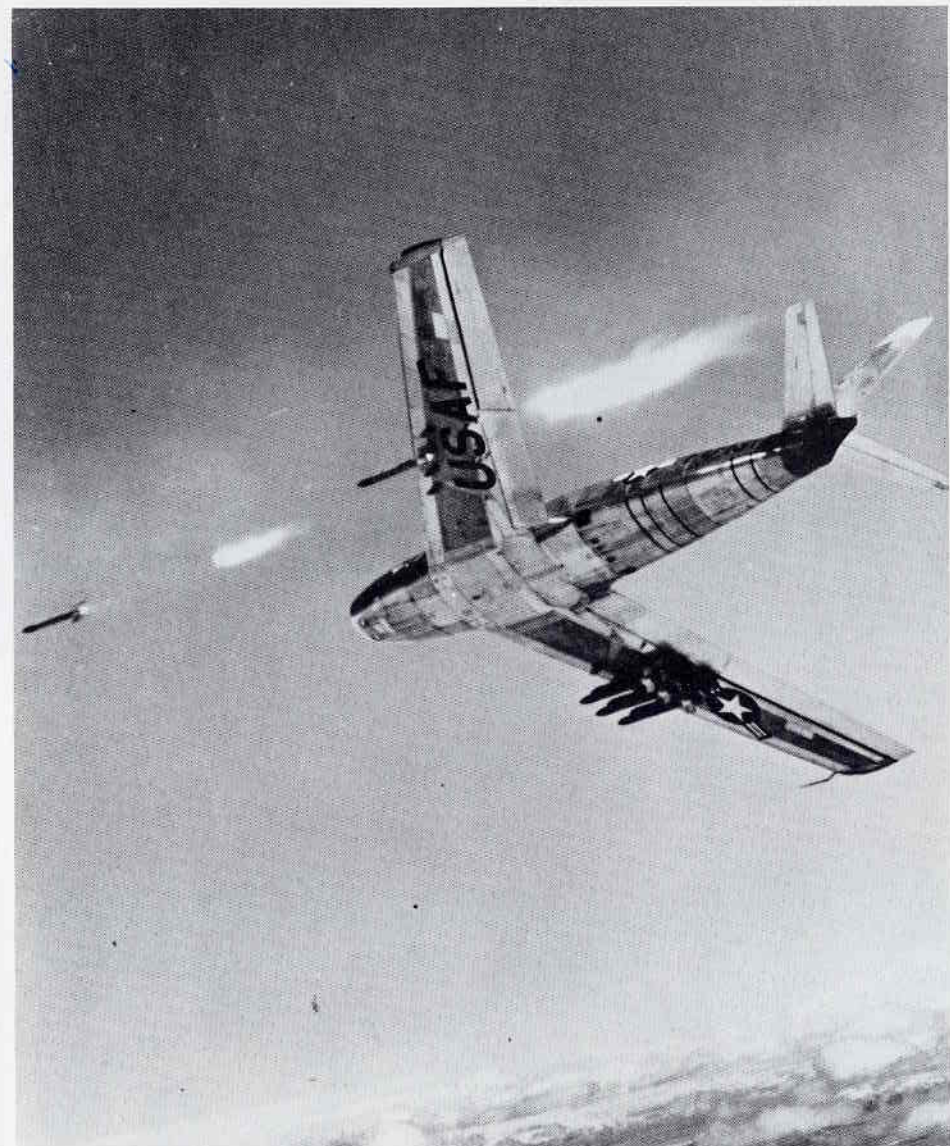
[Center Left & Above] 49-1131 was used by Air Training Command to test use of 5 inch rockets for ground support role, firing rockets, showing the launchers. [NAA]
