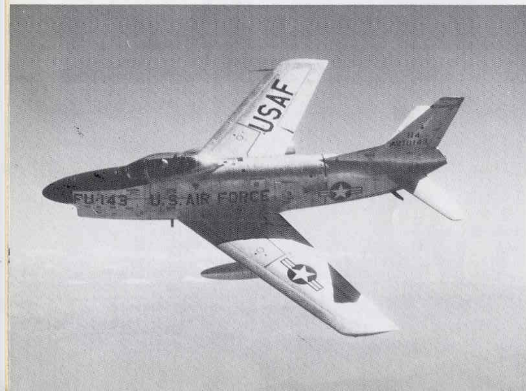
52-10143 is an F-86L-50. Note the SAGE antenna jutting from the fuselage bottom in front of wing. [NAA]
