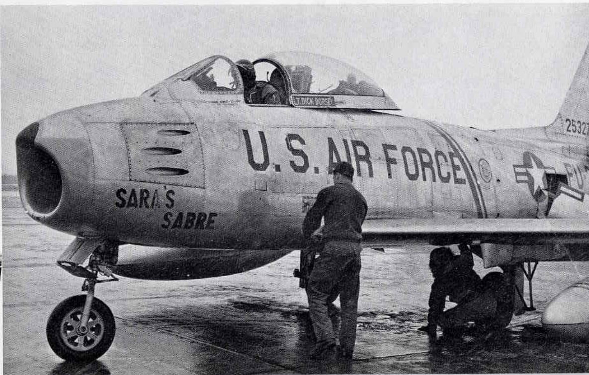
"Sara's Sabre", #52-5327, served with the 4th FDW. Note the inboard pylons. [AAHS]
