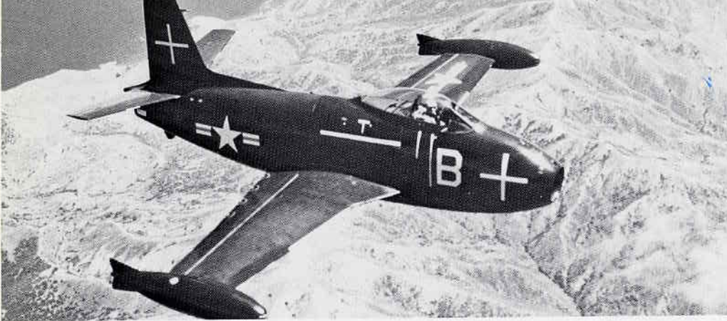
Original XP-86 design was based on the FJ-1 Fury. But the straight-wing design would not allow the 600 mph speed that Air Force wanted. [NAA]
