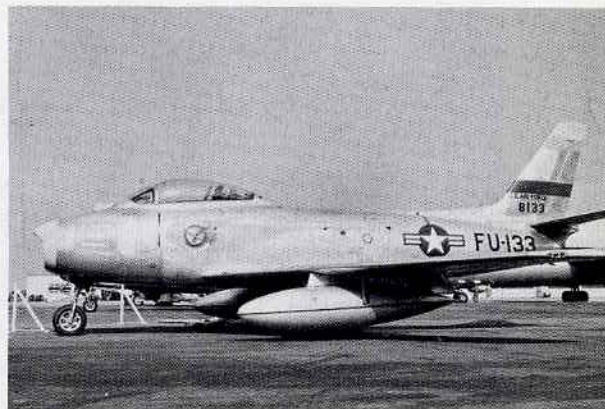
48-133 flew with the 27th FS at March AFB. Fuselage flash and upper tail stripe are yellow, lower stripe is red. Note the 206 gallon ferry tanks. [M/Sgt. David Menard]
