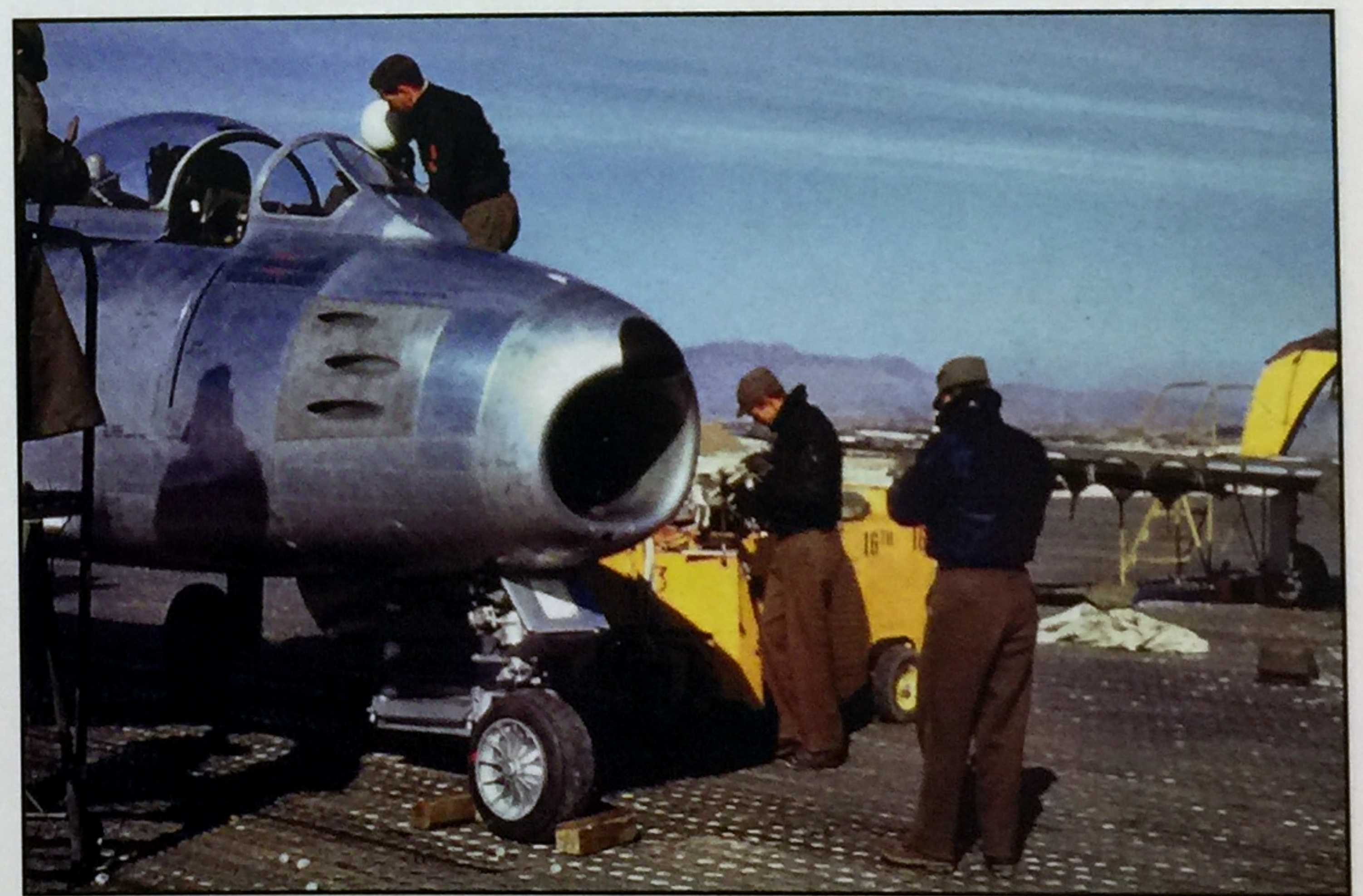
Just as soon as the maintenance crews finish the minor maintenance, the pilots are standing by and ready to strap in. Evidently, this F-86 is being readied for a test hop after the ground crews corrected any of the write-ups from the pilot who last flew it on a mission. This was taken on the 51st Wing’s flight line at Suwon in early 1952. (Dean Juhlin)
